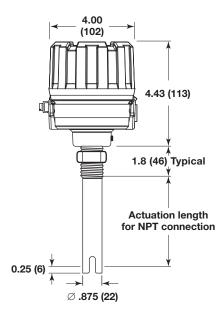
Model 961 with Cast Aluminum Housing and NPT Connection
