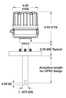
Model 961 with Cast Aluminum Housing and CPVC Flange
