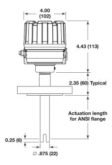
Model 961 with Cast Stainless Steel Housing and ASME Flange
