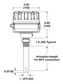
Remote Transducer with NPT Connection
