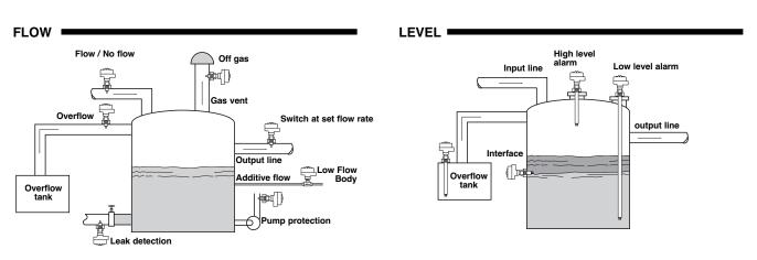
For flow switches calibrated by MAGNETROL, install the probe near the centerline of the pipe. If not calibrated by MAG-NETROL, install the probe at least 1/4 diameter depth into the pipe. For best results it is recommended to install the switch with five diameters of straight run upstream and downstream of the sensor.
