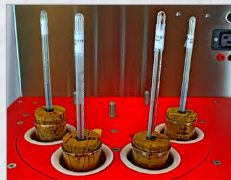
The SBT®+2 tests four (4) Cloud & Pour Point samples at a time. Accessories used with this Insert Module include Copper Sleeves, Glass Stators, Cork Rings & Discs, and Test Jar Stoppers.
