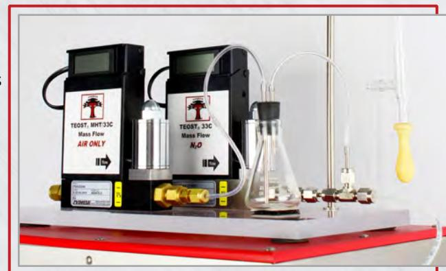
Tannas offers two TEOST® Mass Flow Controller models. The MHTurbo® Mass Flow Controller operates with the D7097 and D8447 tests, while the 33C Mass Flow Controller is utilized for all three TEOST tests (D6335, D7097, & D8447). Contact Tannas Co. for more details on these new Mass Flow Controller systems.
